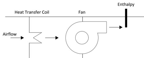
Fig. 1. A simplified field test setup – The exhausted airflow heat gets extracted and this energy is then transferred to the systems supply fan incoming outside air needed for proper design ventilation.
