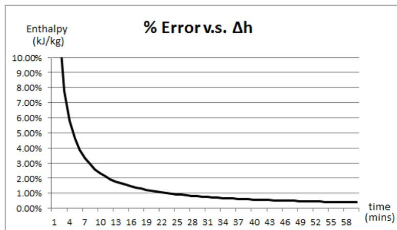
Fig. 4. The airflow error percentage converges to less than one percent for a delta enthalpy above 23.24 kJ/kg when experiencing a 0.23 kJ/kg variation over time.
