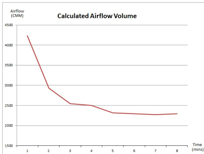
Fig. 3. Using the time stepped enthalpy method the airflow volume is calculated and plotted. Identified, the system reaches steady state where the airflow converges at 2265 CMM.
