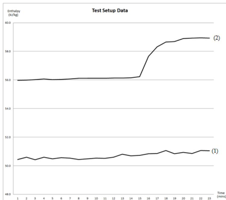
Fig. 2. The test setup data identifies the increasing outdoor enthalpy over time in the graph labeled one and the time-stepped enthalpy method in graph labeled two.
