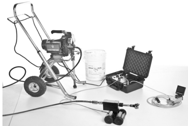
Figure 4.4: A typical HVAC robotic system setup.
