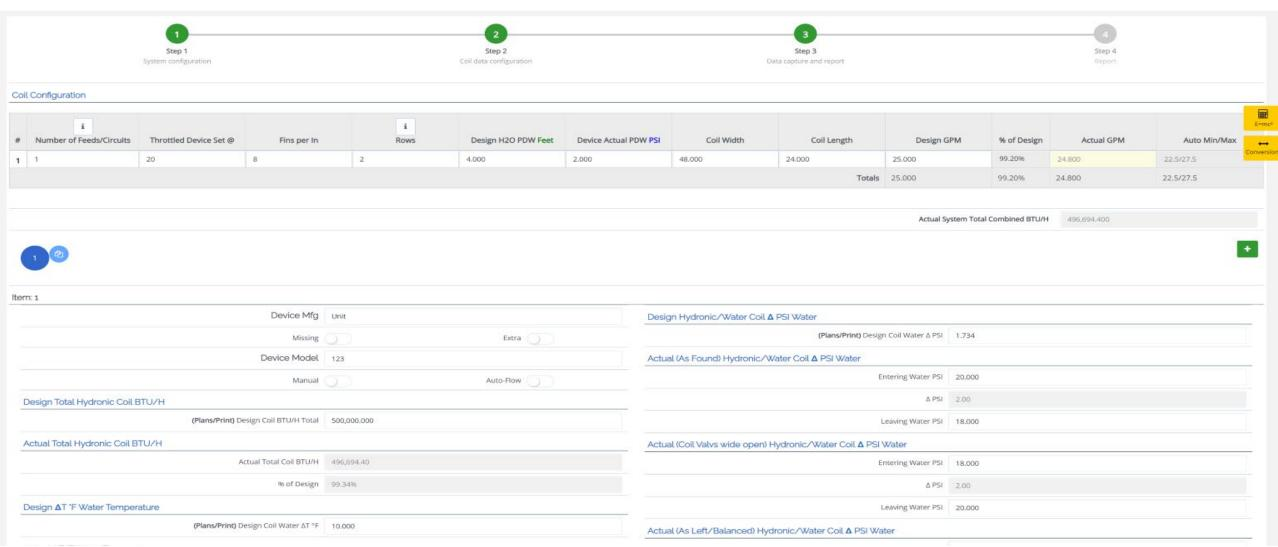
If a calibrated balancing device is selected, this box will appear.
